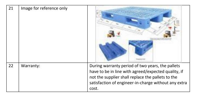
Note: These Pallets will be used in ambient temperature as well as Cold chambers where the working temperature will vary between 2 Deg to -6 Deg C.
